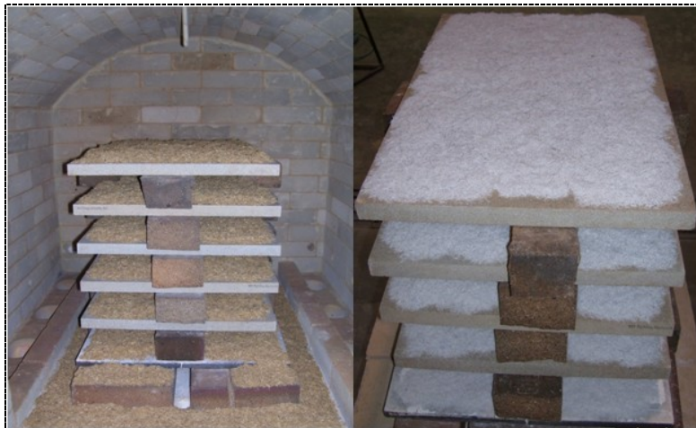
Fig. 1. Rice husk ash in Gas Furnace before (left) and after burning (right)
