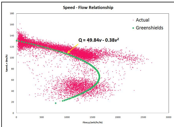
Figure 6. Speed-flow model using Greenshields
