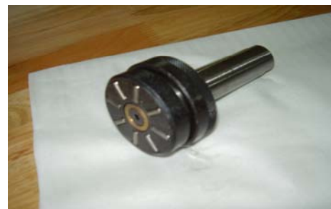
Figure 2: Multi-roller burnishing tool
