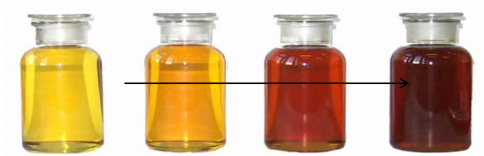
Figure 2.4: Degradation of oil insulation from left to right
