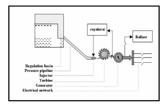
Figure 1.3: Synoptic diagram of a MHPP.
