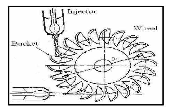
Figure 1.4: The geometrical shape of a Pelton turbine.
