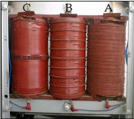
Fig. 3 Prototype Transformer Winding
