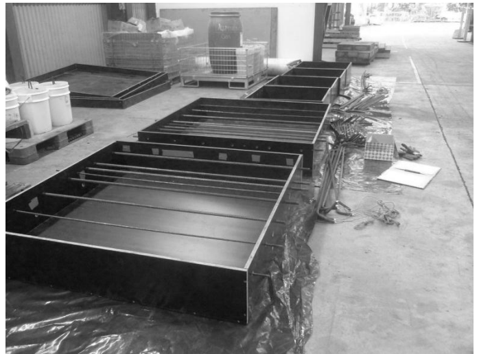
Figure 13. Additional six specimens for the second stage of the accelerated corrosion test.
