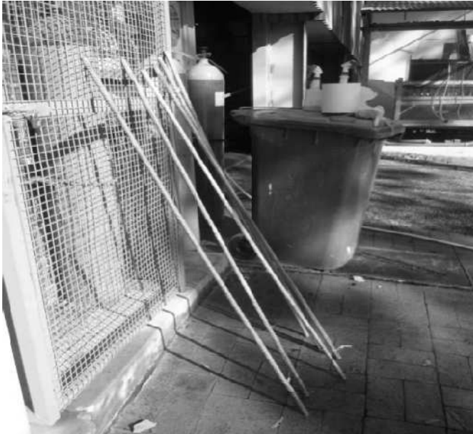
Figure 8. Gravimetric weight loss method: Reinforcing bars were rinsed with methylated spirits and acetone for rapid aeration.
