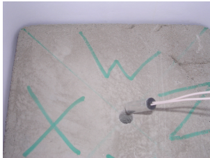
Figure 2: Detonator charge insertion
