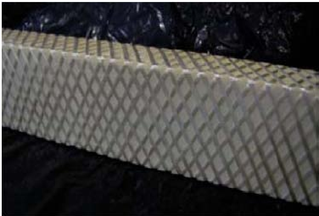
Figure 2.3: Foam board strip wrapped by fiber glass fabric (Stoll et al. , 2004)
