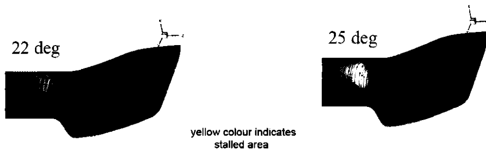
Figure 2.12: CFD Results for the flow separation near the notch region of a BERP blade.
