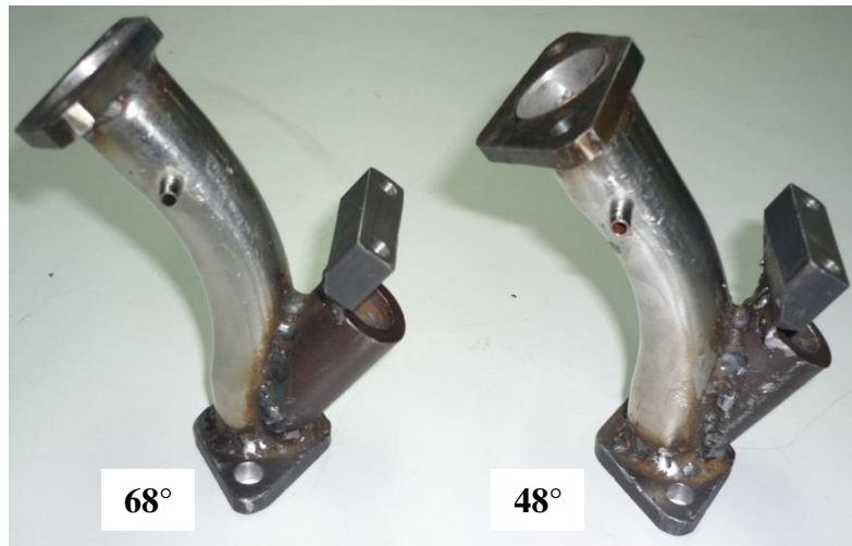
FIGURE 3. Fabricated intake manifold with different fuel injector angles.
