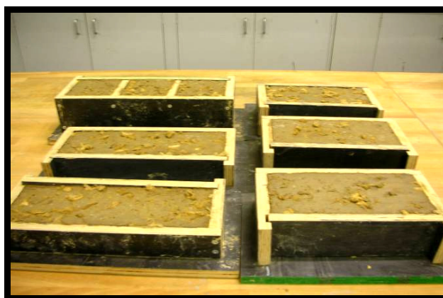
Figure 1 : Compacted Bricks, Beams and Cubes (Clay-CBs mix)
