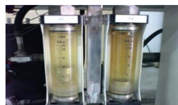
Fig. 2 The cold and hot flow rates measurements of four heat exchanger types model HE158C.
