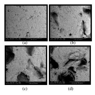
Fig. 1 Electron micrographs images at 100X magnification for different percentages of CBs incorporated into fired clay bricks: (a) 0% CB content (b) 2.5% CB content (c) 5% CB content (d) 10% CB content.
