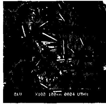
Figure 2. Fracture surface of 2.5 % fiber volume fraction at 50°C fiber
