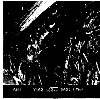
Figure 6. The fracture surface of the 20% fiber volume fraction reinforced composites at 100°C
