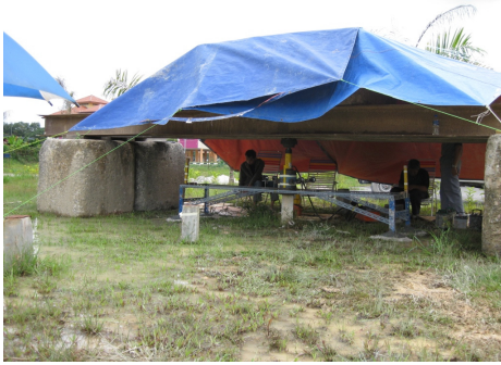
Fig. 3: S-M pile loading test is underway
