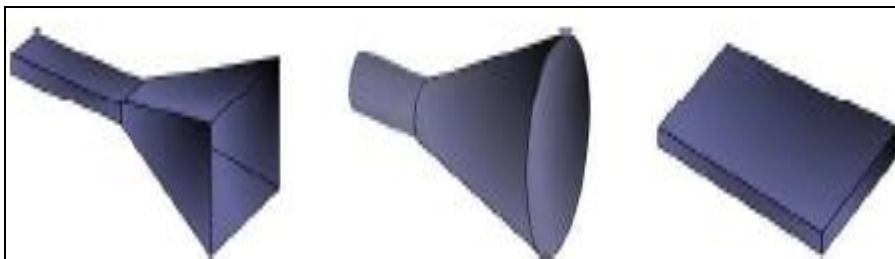
Figure 2.5: Aperture Antenna Configurations. From left to right, pyramidal horn, conical horn, and rectangular waveguide. (Balanis, 1997).
