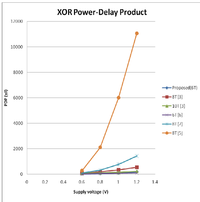
Figure 10. Power-delay products (PDP) of different XOR circuit
