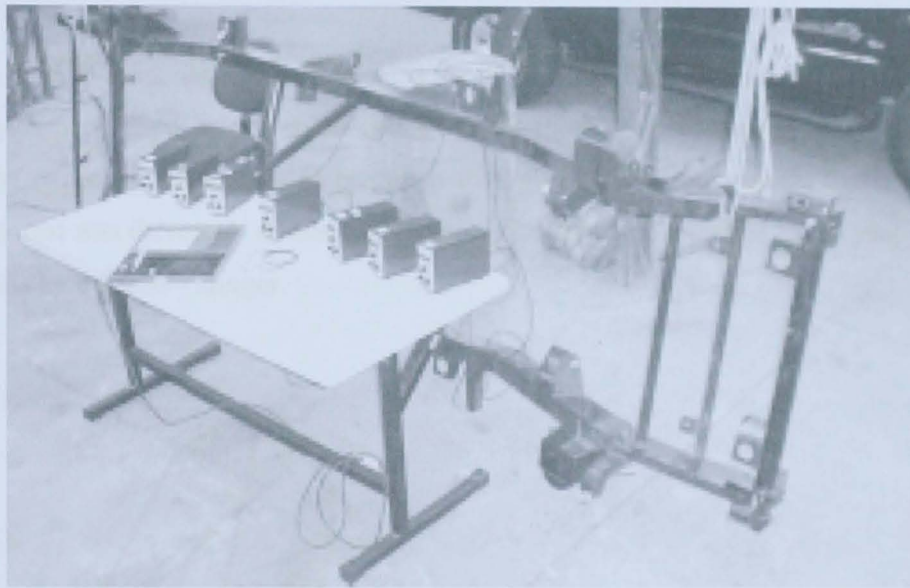
Figure 2.1: Experimental modal analysis setup for truck chassis [1]
