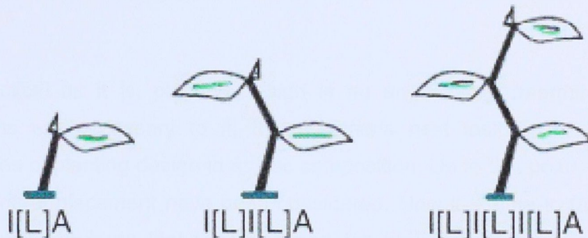
Figure 4: Consecutive stages of development of a plant modeled by a simple L-system with production rule A \rightarrow I[L]A . The structure is represented by a string of characters that changes over time. I stands for an internode, L represents a leaf and the apical meristem is symbolized by A. (source: Renton et al., 2005)
