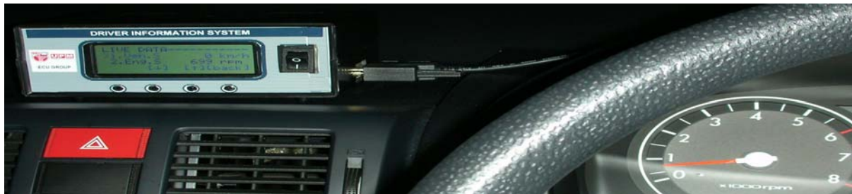
Figure 6: Proposed DIS is interfaced with Hyundai Getz car's ECU
