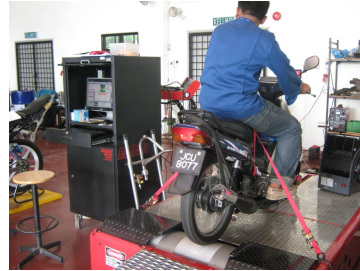
Fig. 2. Performance test conducted on motorcycle chassis dynamometer.
