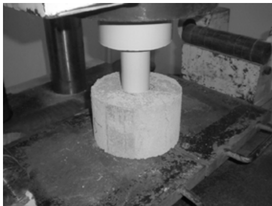
Figure 19. 50mm size of indenter
