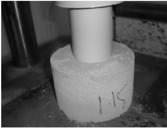
Figure 20. 70.5mm size of indenter
