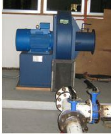
Fig. 2: A blower (left) and a test section containing a PAZ filter (right)
