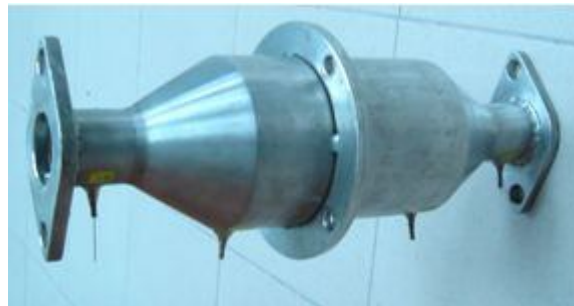
Fig. 3: PAZ filter installed inside the casing
