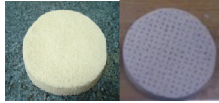
Figure 2. Porous monolith (left) and channelled porous monolith (right)
