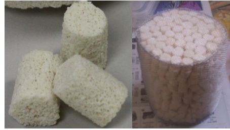
Figure 3. Cylindrical beads (left) and cylindrical beads arranged in the casing (right)
