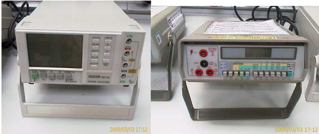
Figure 7: (a) The Power Analyzer DIGICON (DW-735) (b) The Digital Multimeter GW (GDM-8034)
