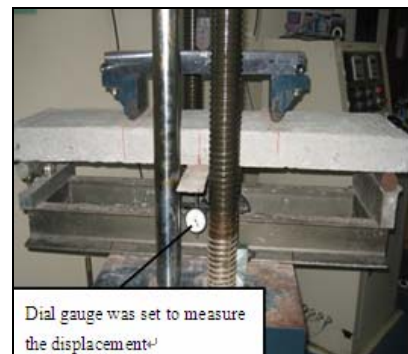
Figure 4: Four-points bending test setup
