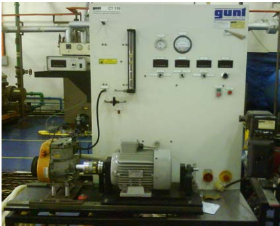
Fig. 4. Engine test rig based on GUNT asynchronous dynamometer.
