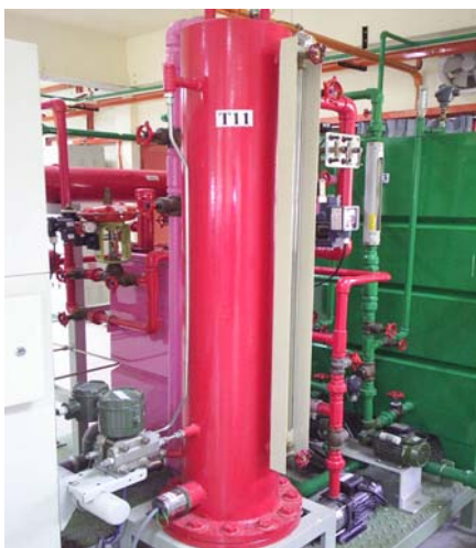
Figure 4 - The real system of boiler drum QAD Model BDT 921
