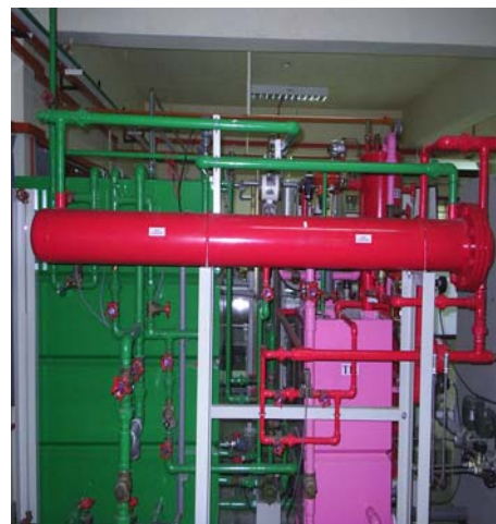
Figure 7 - The real system of heat exchanger QAD Model BDT 921
