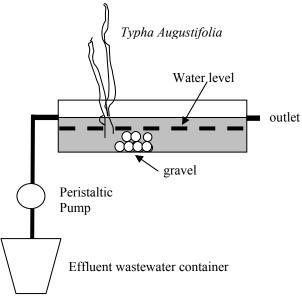
Fig.1 A schematic diagram of the SSF Constructed Wetland
