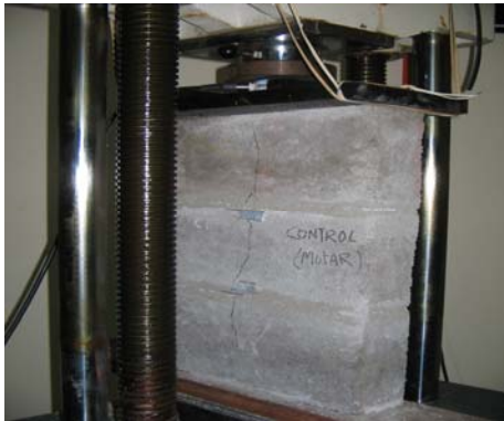
Figure 6: Vertical splitting Failure Of Control Cement Block Prism
