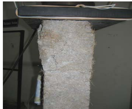
Figure 7: Bulging Failure of EFB fibre cement Block Prism.
