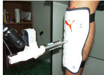
Figure 3. LVDT attached to the modified shin pad.
