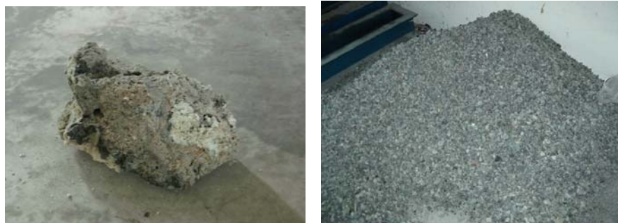
Figure 1: Lightweight Palm oil clinker obtained from palm oil mill (left) Pile of crushed palm oil clinker aggregates (right)
