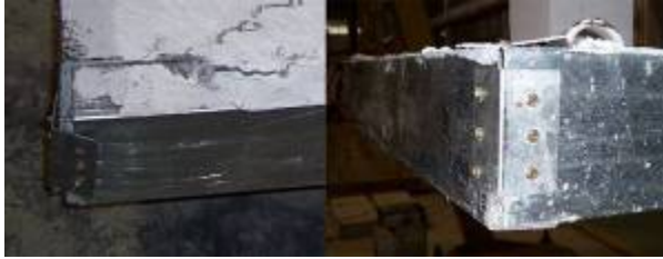
Figure 7 – Failure observed in experimental test, bracket torn off (left) and edge expansion (right).
