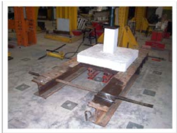
Figure 4 – Setting of specimen on test rig to test for shear/moment (above) and test for punch (lower).
