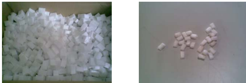
Figure 1: Original cut Styrofoam aggregates (left) oven-dried Styrofoam used (right)
