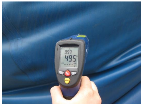
Figure 4.7. The temperature of the balloon is measured with an infrared thermometer.
