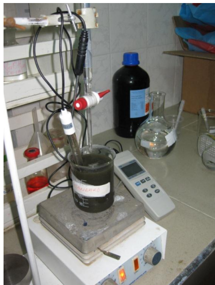
Figure 4.13. Setup of lab equipment for analysis of alkalinity.
