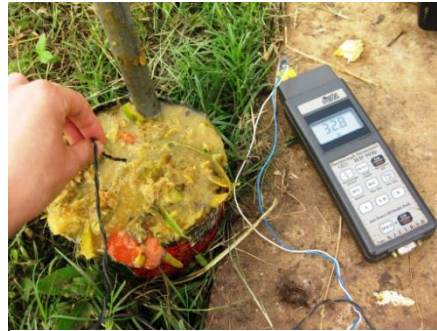
Figure 4.9. The temperature of the influent was measured.
