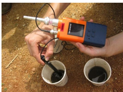
Figure 4.11. pH of digestate was measured.
