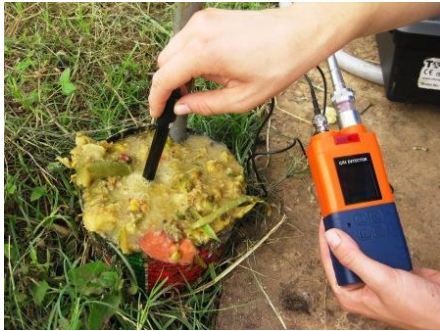
Figure 4.8. The pH of the influent was measured with a portable pH meter.
