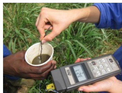
Figure 4.12. Temperature of digestate was measured.
