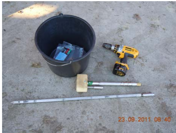
Figure 1. Stickit-drill and extension Photo: Claes Jonsson.
