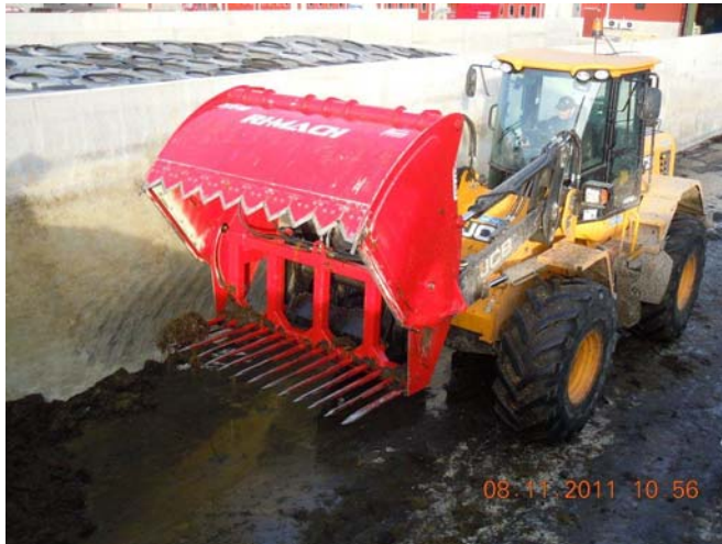
Figure 9. Block-cutter machine used at Lövsta. Photo: Claes Jonsson
