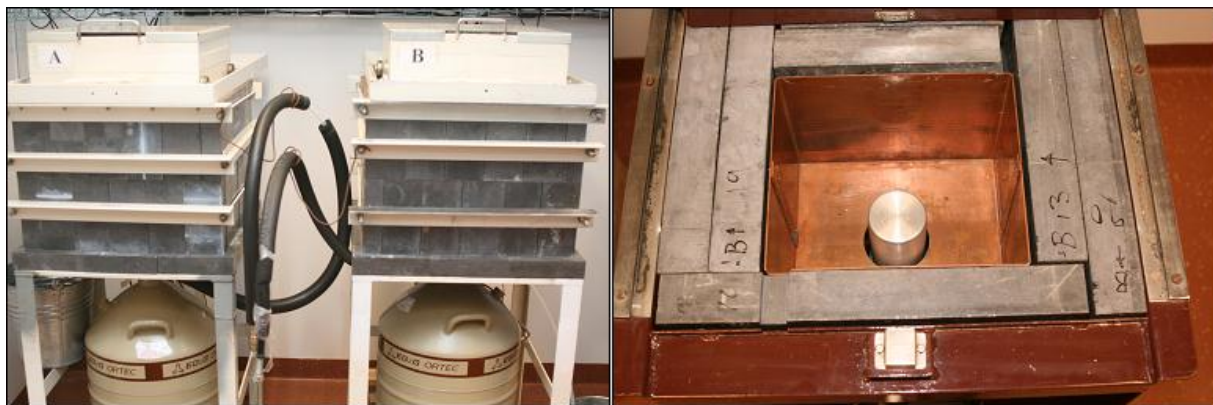
Fig.4 Gamma detectors used for ^{137}\text{Cs} measurement in the animals.
