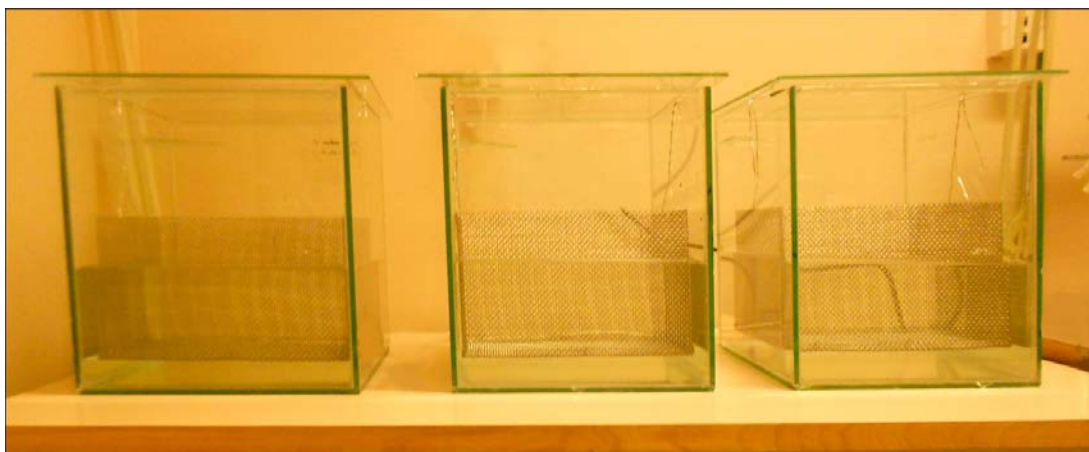
Figure 3a. Design of the uptake experiments, representing the three replicate aquaria
