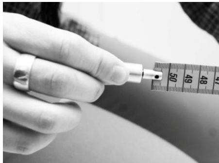
Figure IV: A dynamometer at the end of the tape measure to ensure that the same force is used in each measurement.
