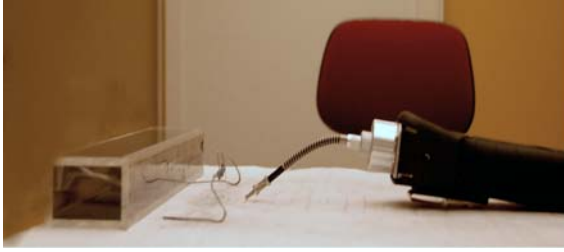
Figure 2. Measurements of plumes with PID in the open-arena olfactometer.
