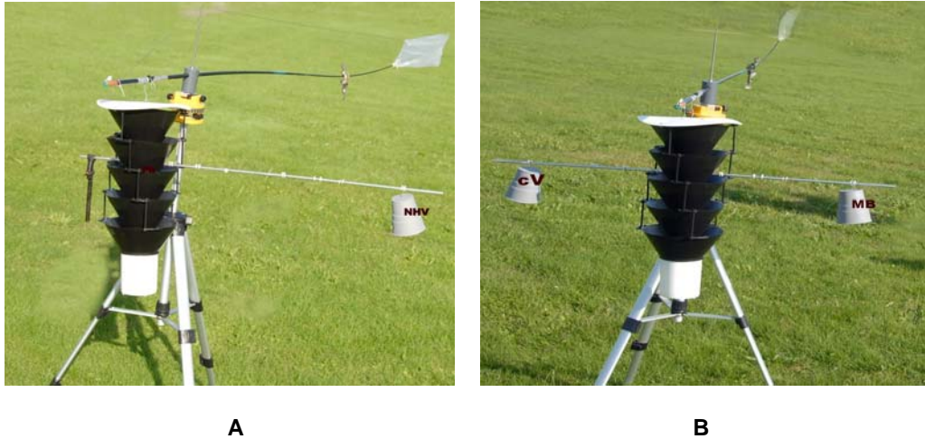
Figure 5. A. Modified Lindgren 5 funnel trap used in horizontal spacing between NHV and pheromone. Pheromone dispenser is in the central funnel and NHV under shady hat. B. Modified Lindgren trap used in horizontal spacing between pheromone components (placed under shady hats). Photo: Muhammad Binyameen
