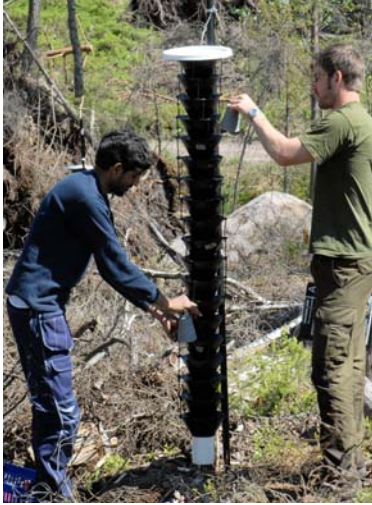
Figure 4. Lindgren 19 funnels trap and changing of dispenser cups in the vertical experiment. Photo: Fredrik Schlyter.
