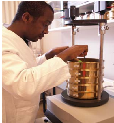
Figure I. Separation of clumped particles during the dry sieving process. (Photo by Elise Bostad)
