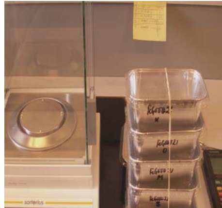
Figure II. Different sieving fractions of the sample in pre-weighed aluminum containers. (Photo by Elise Bostad)
