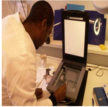
Fig III. Separation of particles on scanner. (Photo by Elise Bostad)
