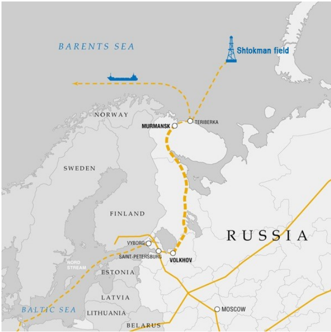
Figure 12. Murmansk-Volkhov gas pipeline (Gazprom, 2011e).
