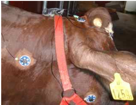
Figure 2. Attachment of surface electrodes for electrophysiological recordings on dairy cows; ground electrode (EEG), right eye electrode (EOG) and right neck muscle electrode (EMG).
