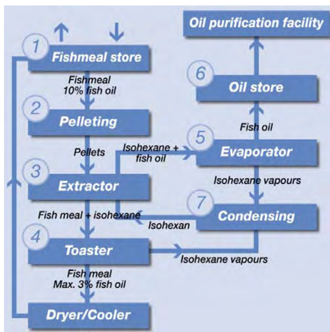
Figure 4. Fish meal extraction scheme. ( www.999.dk )
