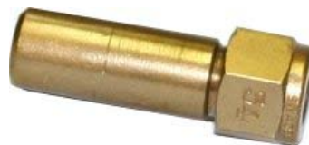
Figure 3. SF 6 permeation tube introduced in cow's rumen.
