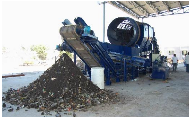
Figure 20 Segregation unit for separation of the organic and inert components. [37]
