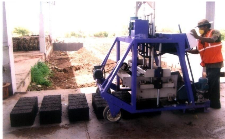
Figure 25 The mechanical processing of bricks. [37]
