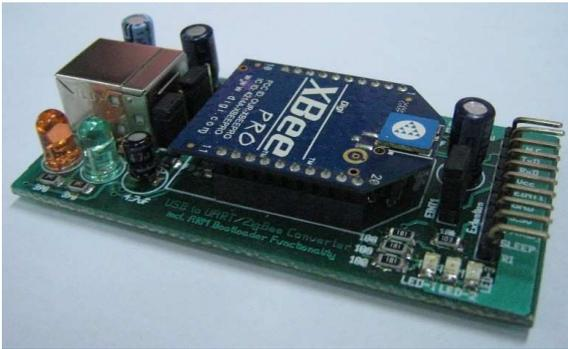
Gambar 4. USB to ZigBee Converter
