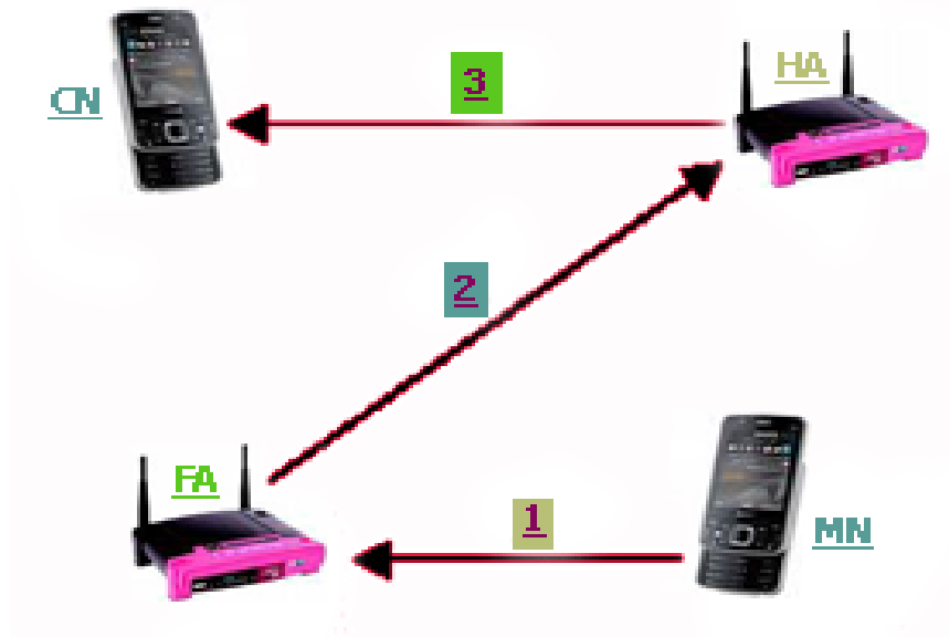
Figure 2.20: The MN sends packets to CN via foreign network
