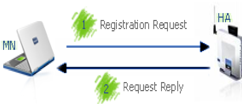
Figure 2.18: The MN directly registers its current location through the HA in Mobile IPv6
