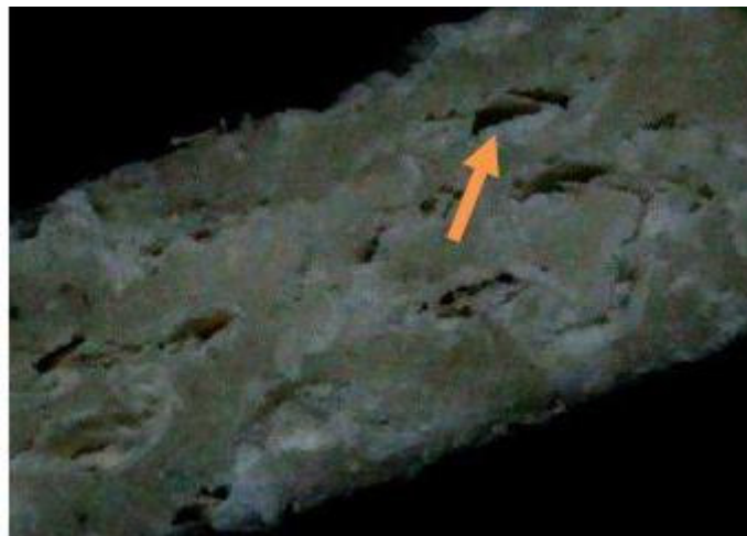
Figure 4: Cross section of single coated epoxy syntactic foam after compression
